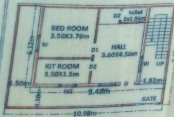
GROUND FLOOR-PLAN [Scale-1cm=1.00m]
